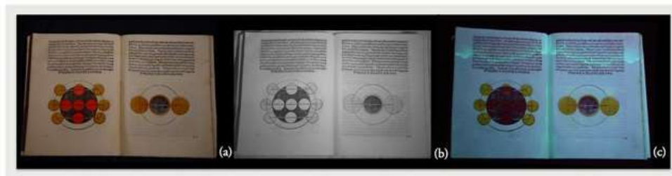
Figure 12: Imaging in Visible Light (a), IR (b) and UV fluorescence (c) of a 1485 Venetian printed book. (Data from [18])
